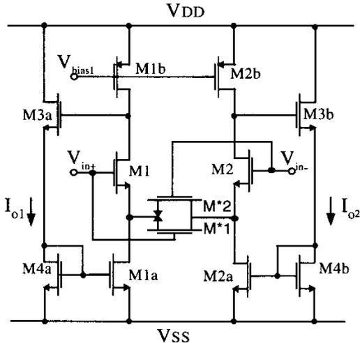
Fig. 3. The highly linear V-I converter
