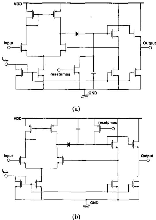
Figure 5. Peak detection circuits (a) top hold circuit and (b) bottom hold circuit.
