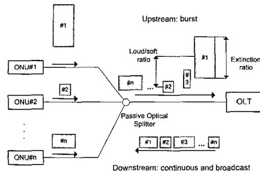
Figure 1. Architecture of general PON system
