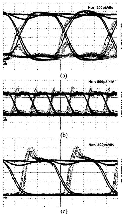
Figure 9. Eye diagrams of the transmitted power over temperature with/without the feedback. (a) and (b) are lower and higher temperature with the feedback, respectively, and (c) is without the feedback.
