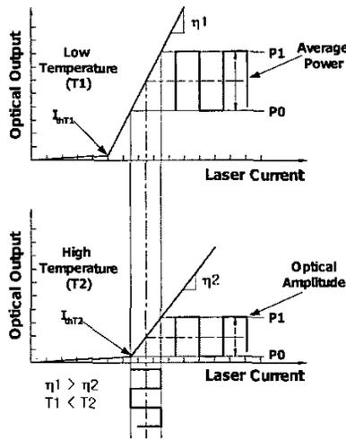
Figure 2. Temperature characteristics of a laser-diode as an optical output vs. laser current.
