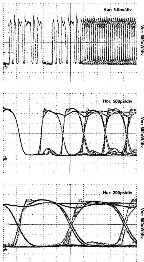
Figure 8. Eye diagrams of one of the two bursts shown in Figure 7t the room temperature.
