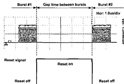
Figure 7. Measured waveforms for 1.25Gb/s burst mode with  $2^9 - 1$  PRBS data
