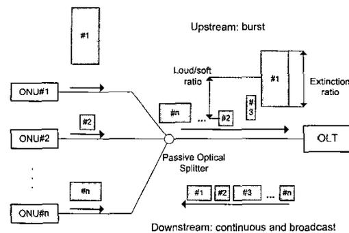
Figure 1. Architecture of general PON system
