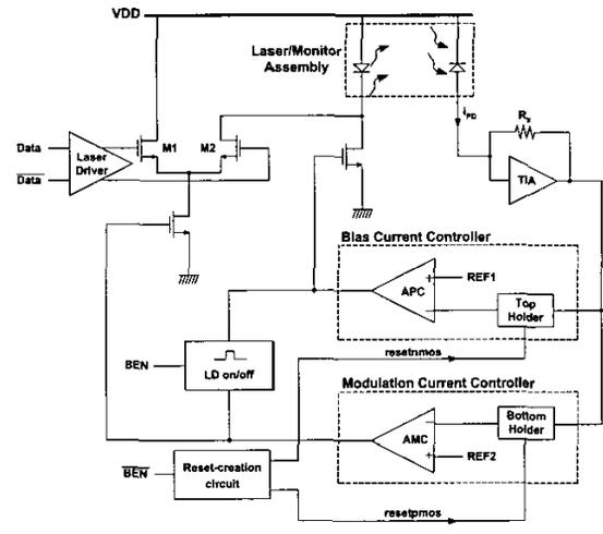
Figure 3. Block diagram of the proposed transmitter architecture with temperature compensation for laser-diode.
