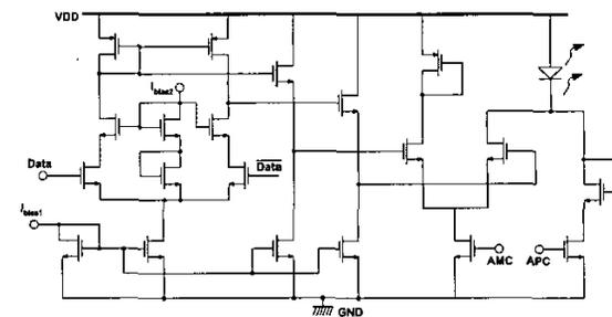
Figure 4. Simplified Laser driver schematic.
