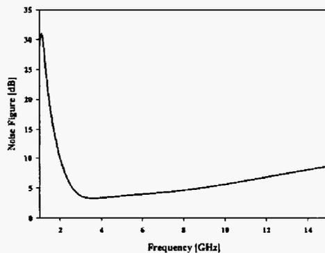
Figure 4. Simulated noise figure of the proposed amplifier.
