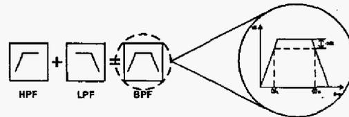
Figure 1. Frequency response of BPF with combination of that of HPF and LPF, respectively.
