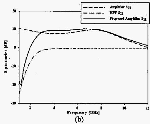
Figure 3. Simulated of  $S_{11}$  and  $S_{21}$  for HPF, the cascode amplifier, and the cascode amplifier combined with HPF, respectively: (a) input return loss ( $S_{11}$ ) and (b) frequency response characteristics ( $S_{21}$ )
