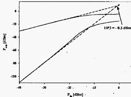
Figure 5. Simulated two-tone test of the proposed amplifier.
