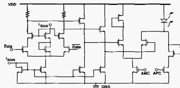
Fig. 5. Simplified Laser driver schematic.
