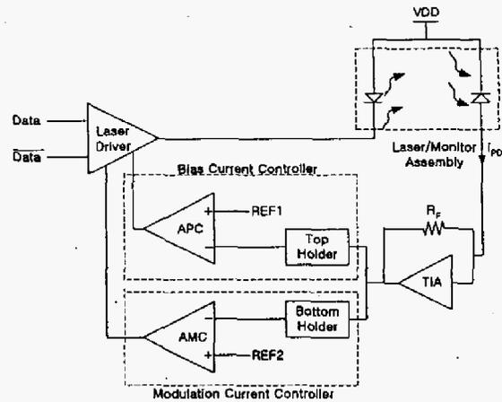
Fig. 4. Block diagram of the proposed transmitter architecture with temperature compensation for laser-diode.
