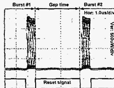
Fig. 9. Measured waveforms for 1.25Gb/s burst mode with  $2^9 - 1$  PRBS
