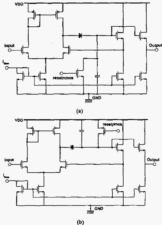
Fig. 7. Peak detection circuits (a) top hold circuit and (b) bottom hold circuit.
