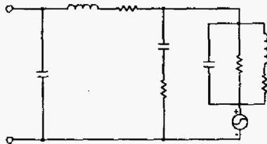
Fig. 6. Small-signal equivalent laser-diode model.
