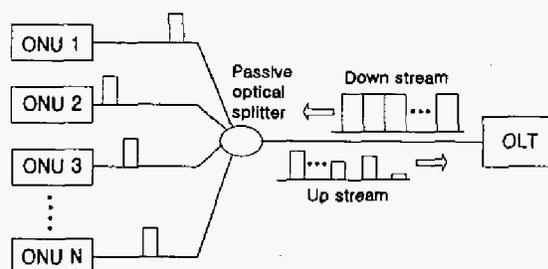
Fig. 1. Architecture of general PON system
