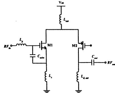
Fig. 4. Schematic of the Driver Amplifier
