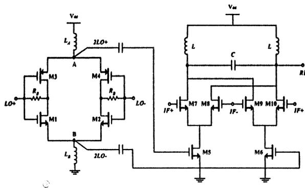
Fig. 3. Schematic of the Up-mixer
