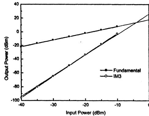
Fig. 6. Linearity of the Driver Amplifier
