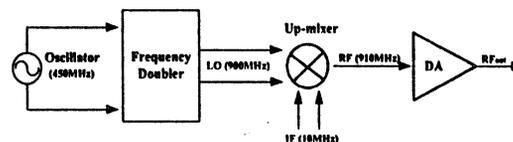
Fig. 1. Proposed Transmitter Front-End
