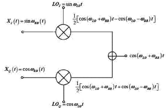
Fig. 6. LSB signal canceling mechanism in IQ path
