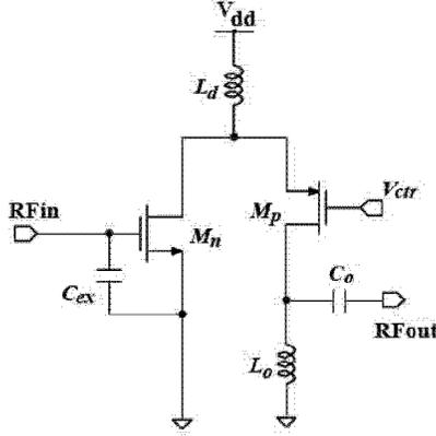
Fig. 3 Schematic of the driver amplifier
