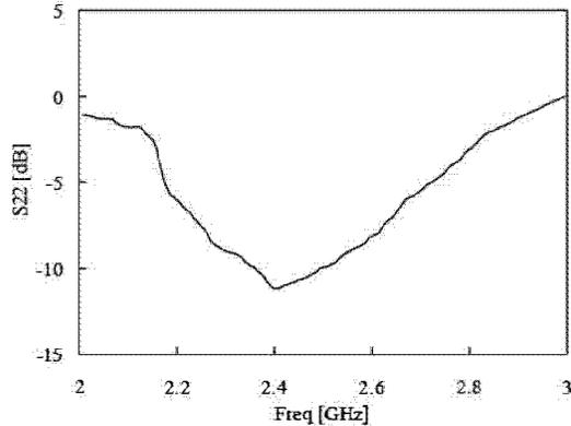
Fig. 8. Measured  $S_{22}$  of the RF transmitter front-end
