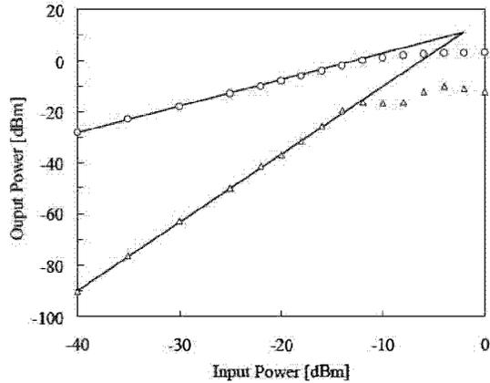
Fig. 7. Measured OIP3 of the RF transmitter front-end at its highest gain mode
