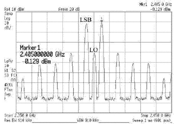
Fig. 5. Measured output spectrum of the RF transmitter front-end at the -12 dBm input power
