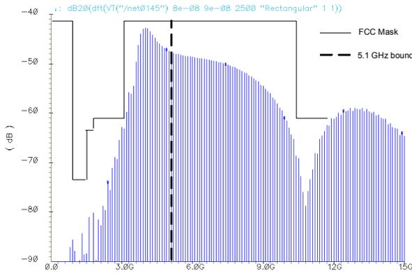
Figure 7. Pulse PSD in compliance with FCC mask
