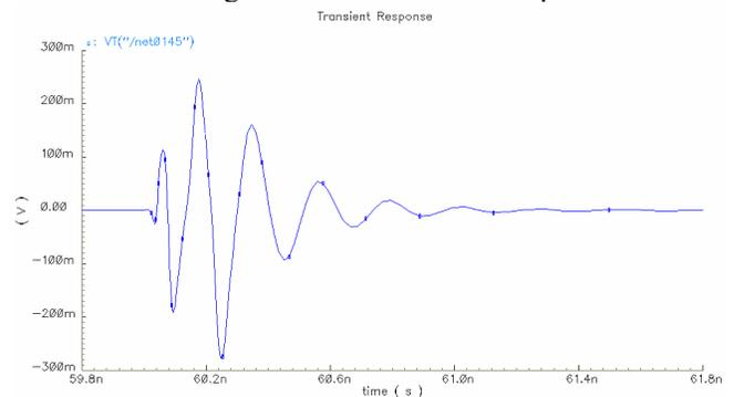
Figure 6. A single 7<sup>th</sup> Derivative Gaussian pulse
