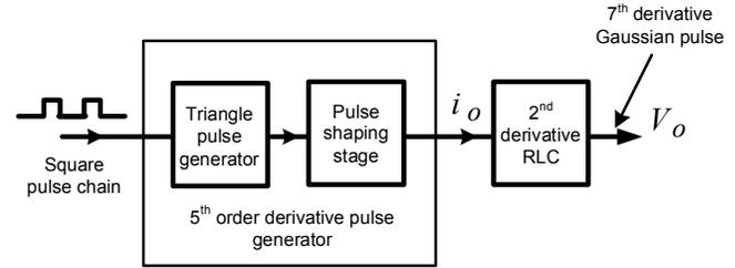
Figure 2. Block diagram of the proposed pulse generator
