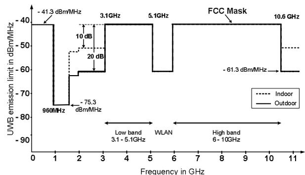
Figure 1. FCC spectrum mask
