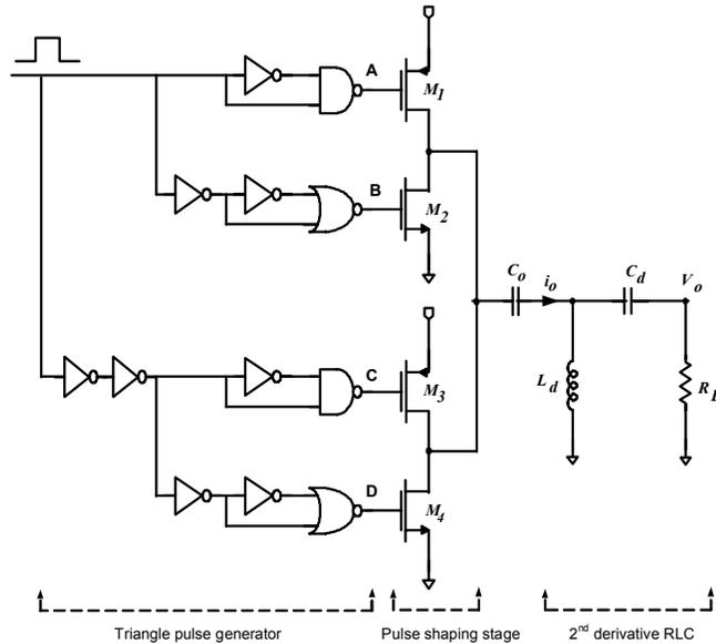
Figure 4. The proposed 7<sup>th</sup> derivative Gaussian pulse generator
