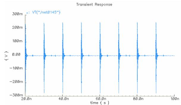
Figure 5. Output pulse chain at 100 MHz PRR
