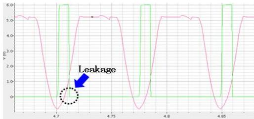
Fig. 3(a). Simulated  $V_{P/N}$  and power switch control signal of conventional rectifier.
