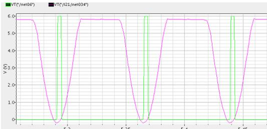
Fig. 3(b). Simulated  $V_{P/N}$  and power switch control signal of proposed rectifier.
