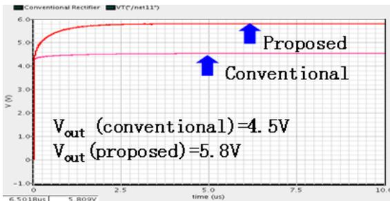
Fig. 4. Rectified output voltage  $V_{REC}$  of discussed rectifiers.
