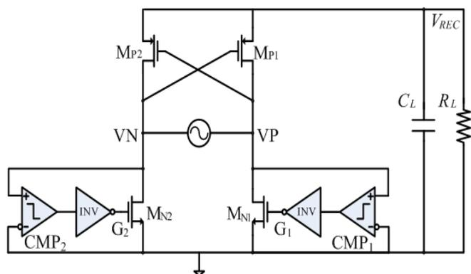
Fig. 1. Architecture of cross-coupled comparator based active rectifier.
