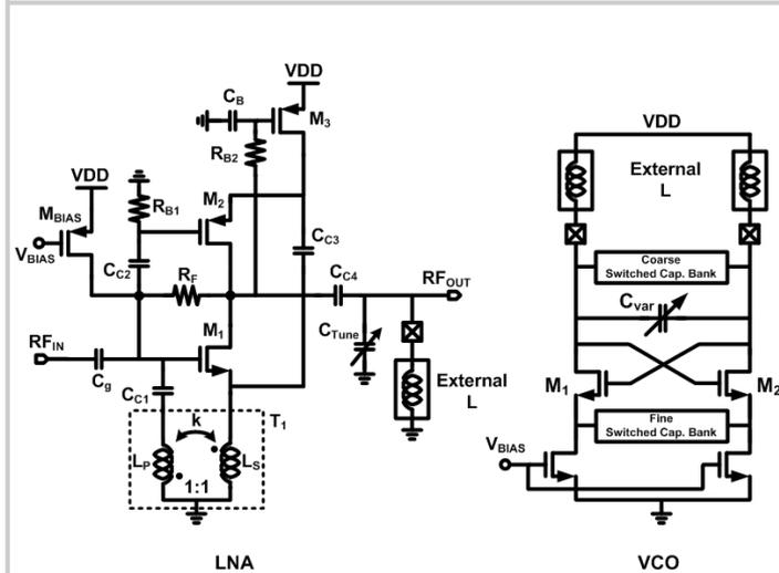
Figure 13.1.3: Schematic diagrams of LNA and VCO.
