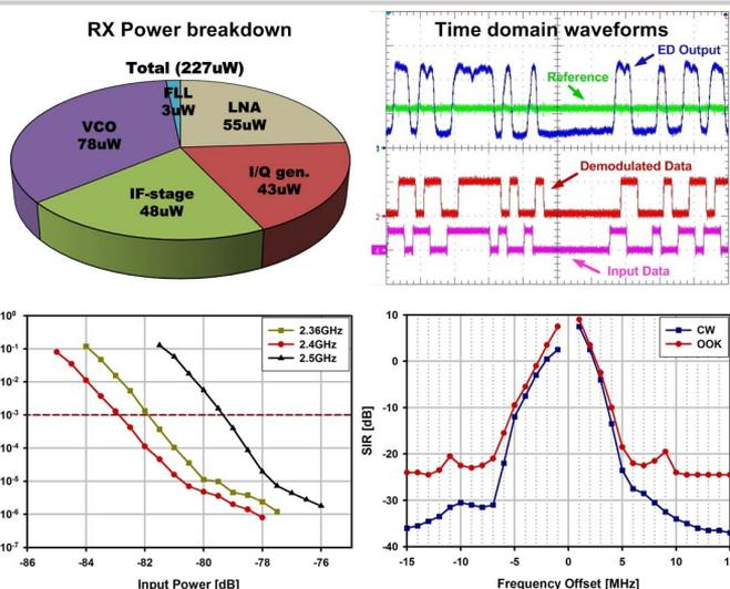
Figure 13.1.4: Power break-down and measurement results of time-domain waveforms, BER, and SIR to CW & OOK interferers.
