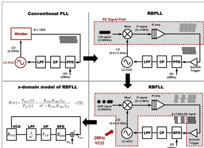
Figure 13.1.1: Block diagram for PLL, RBPLL, RBFLL, and the s-domain equivalent model of RBFLL.
