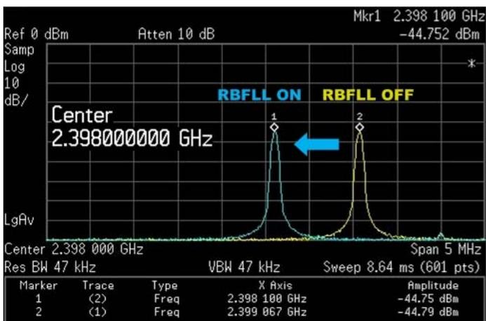
Figure 13.1.5: Measured VCO spectra with RBFLL on and off.
