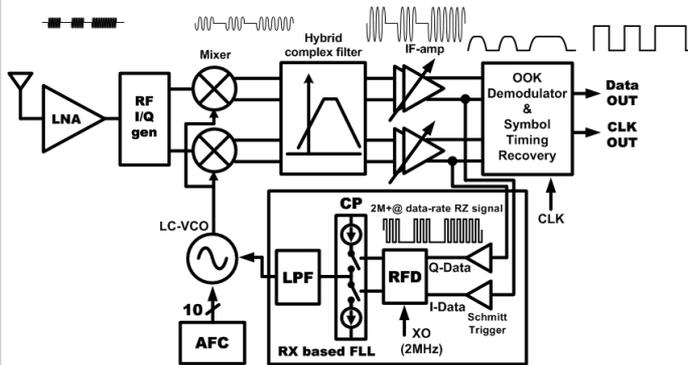
Figure 13.1.2: Overall block diagram of a 2.4GHz multi-channel ULP RX with proposed RBFLL.
