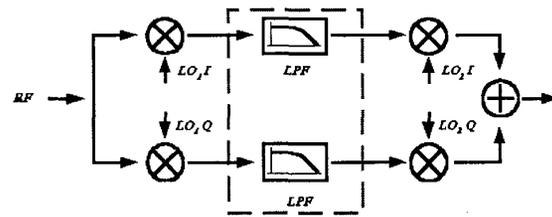
Fig. 2 Weaver Image Rejection Architecture
