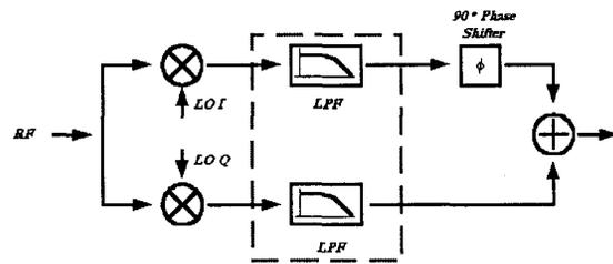
Fig. 1 Hartley Image Rejection Architecture
