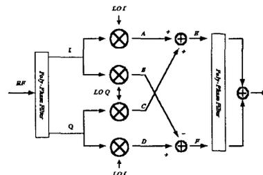
Fig. 3 The proposed Image Rejection Mixer Architecture
