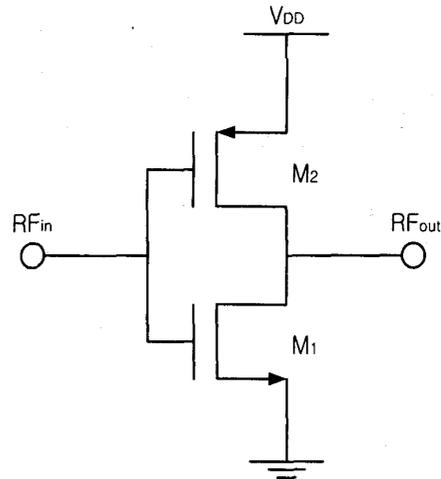
Figure 4. An inverter amplifier.
