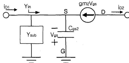
Figure 5. The small-signal equivalent circuit of the 2<sup>nd</sup>-stage of the cascode amplifier.
