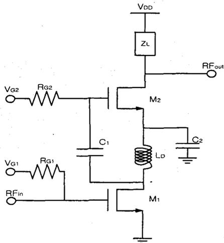
Figure 3. A current sharing two-stage cascode amplifier with inductive 1<sup>st</sup>-stage load.
