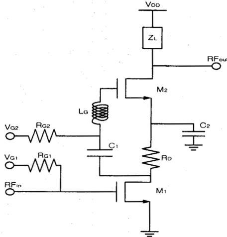
Figure 6. The current sharing two-stage cascode amplifier with a series inter-stage resonance.
