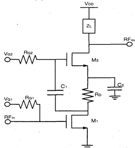
Figure 2. A current sharing two-stage cascade amplifier with resistive 1st-stage load.
