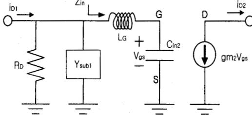
Figure 7. The small-signal equivalent circuit of the inter- and 2<sup>nd</sup>-stage of the proposed LNA architecture.
