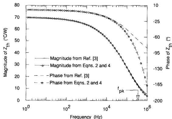
Fig. 2. Magnitude and phase of thermal spreading impedance  $Z_{th}$ . Circled values were computed using (2) and (4); uncircled curves were computed using the Fourier transform of the model in [3].
