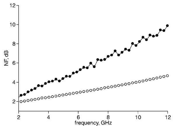
Fig. 3 Measured and simulated noise figure
