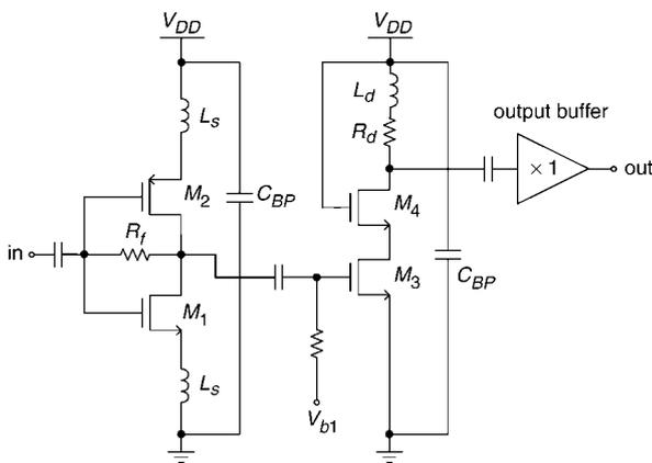
Fig. 1 Circuit schematic of proposed LNA
