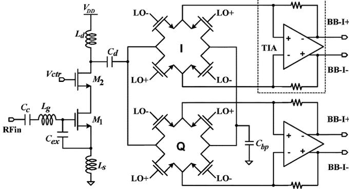
Fig. 2. Schematic of the RF receiver.
