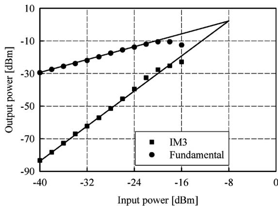
Fig. 10. Measured IIP<sub>3</sub> of the RF receiver front-end.
