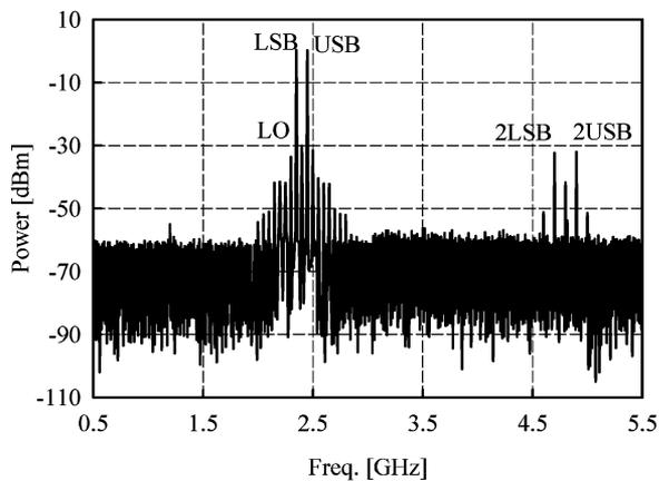
Fig. 11. Output spectrum of the RF transmitter front-end with  $-12$ -dBm input power.
