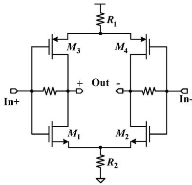
Fig. 4. Schematic of the inverter used in a TIA synthesizer system.
