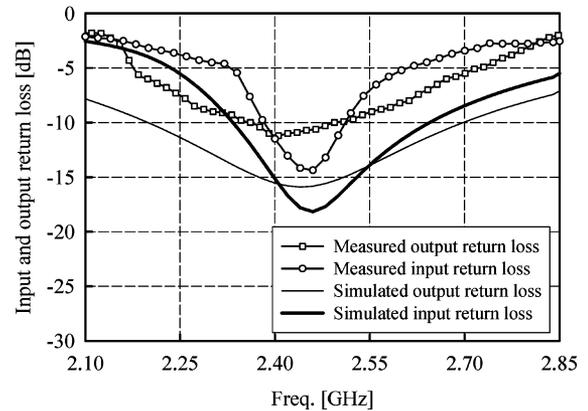
Fig. 8. Measured and simulated input return loss of the receiver and output return loss of transmitter front-end.
