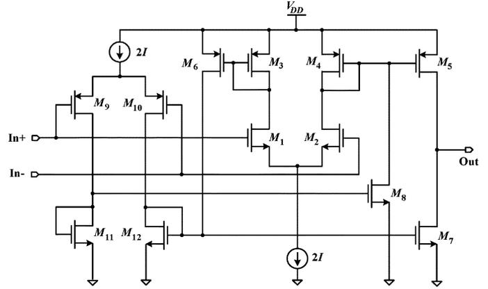
Fig. 5. Schematic of the operation amplifier used in the TIA.
