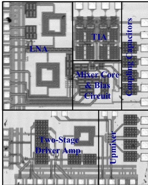
Fig. 7. Microphotograph of the proposed RF receiver/transmitter front-end. (Color version available online at <http://ieeexplore.ieee.org>.)
