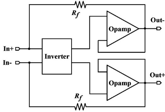
Fig. 3. Block diagram of the proposed TIA.
