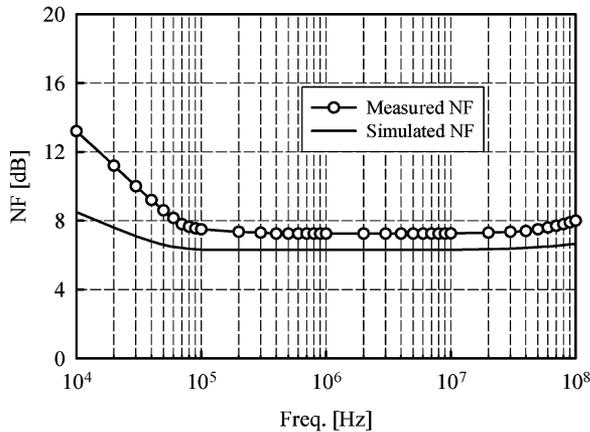
Fig. 9. Measured and simulated NF of the RF receiver front-end.
