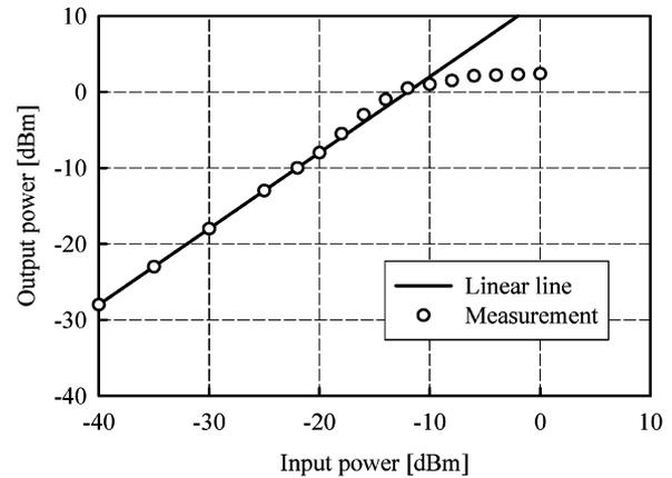
Fig. 12. Measured output 1-dB compression point of the RF transmitter front-end.
