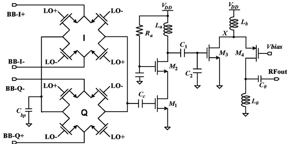
Fig. 6. Schematic of the RF transmitter.
