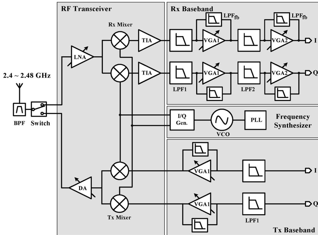
Fig. 1. Transceiver architecture.
