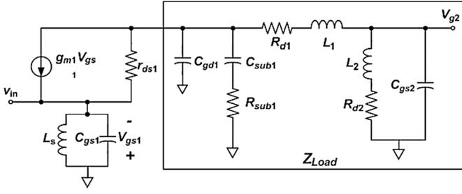
Fig. 2. Small-signal equivalent circuit for the common-gate stage including the load and the parasitic at the drain.
