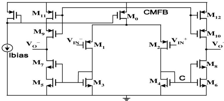
Figure 3. The current mirror OTA with self-cascoding output stage.
