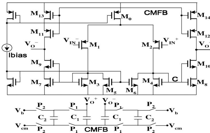
Figure 4. The proposed gain boosted self-cascoding current mirror OTA.
