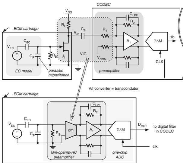
**Fig. 1** Traditional ECM + CODEC configuration (upper) and proposed digital ECM architecture (lower)
