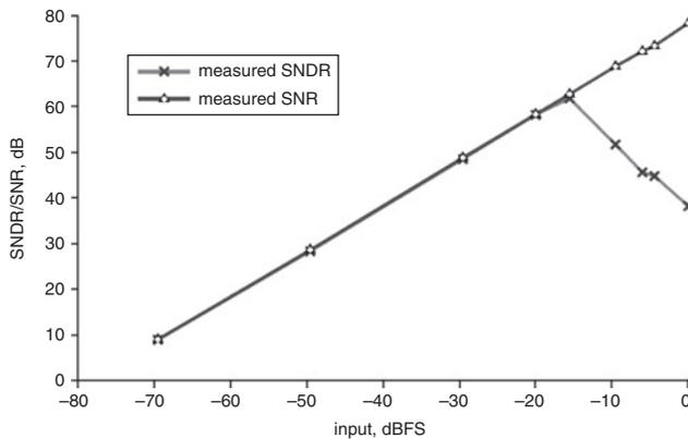
Fig. 4 Measured SNR and SNDR against input level
