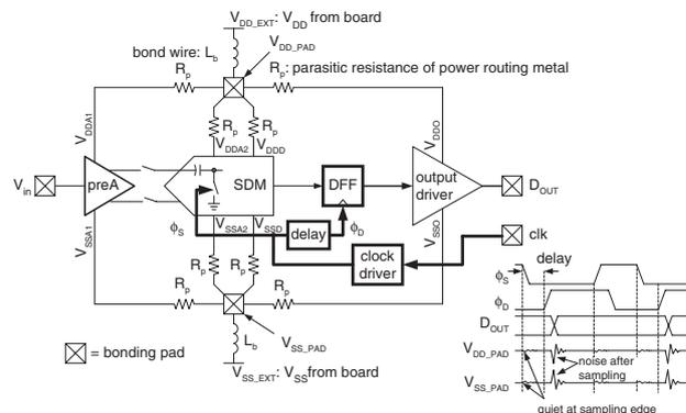
**Fig. 2** Block diagram of prototype with power/ground routing and concept of time-domain noise isolation
