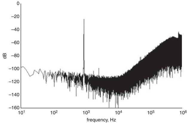
Fig. 3 Measured ADC output spectrum with 1 kHz 30 mV<sub>pp</sub> (-20 dBFS) sinusoidal input signal
