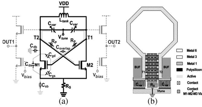
Fig. 2. (a) Circuit schematic of a differential LC-VCO with two buffers. (b) LC-VCO layout with the proposed cross-coupled transistor structure.
