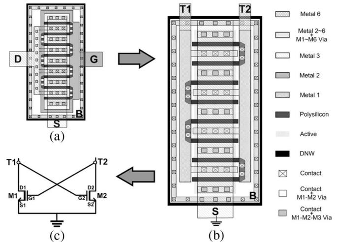
Fig. 1. Conversion of an RF transistor structure. (a) Conventional RF transistor layout, (b) proposed cross-coupled transistor layout, and (c) the corresponding cross-coupled transistor circuit schematic.
