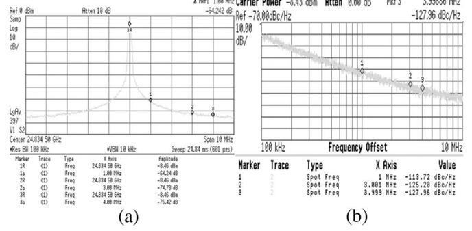
Fig. 3. (a) Measured frequency spectrum. (b) Phase noise of the proposed-transistor-structure-based VCO operating at 24.8 GHz.
