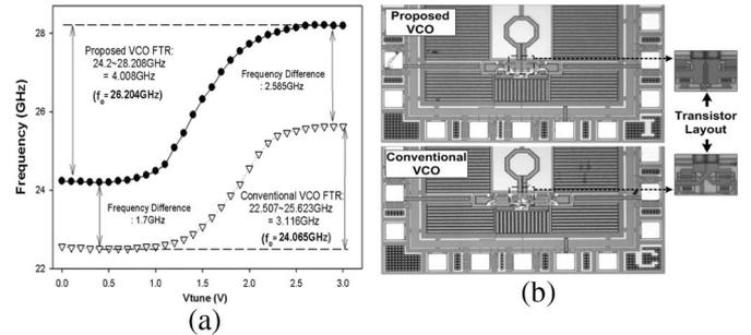
Fig. 4. (a) Measured oscillation frequency versus the control voltage  $V_{tune}$  of the two VCOs using the conventional and proposed transistor structures. (b) Microphotograph of the two VCO chips with the proposed and conventional cross-coupled transistor structures.
