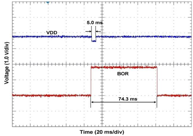
Fig. 7. Measured output reset waveform with a 0.3-V drop of supply voltage ( $V_{low} = 1.5$  V) in  $T_{int} = 5$  ms.
