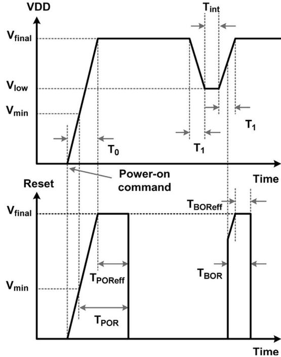
Fig. 1. Timing of POR and BOR.
