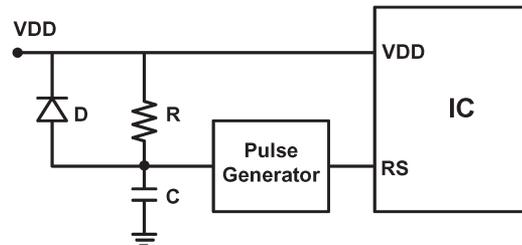
Fig. 2. External POR circuit.
