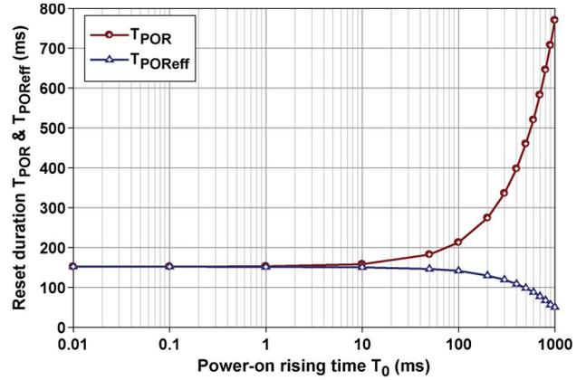
Fig. 6. Measured reset time with respect to the rising time of a power-on event.
