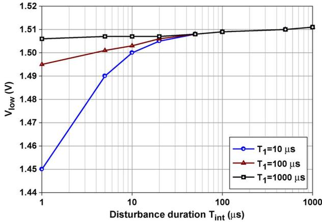
Fig. 8. Measured brown-out detection level versus the duration of a brown-out event.
