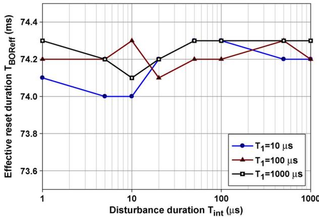
Fig. 9. Measured effective reset time with respect to duration of a brown-out event.
