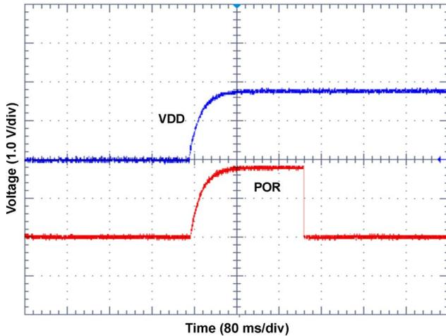
Fig. 5. Measured POR reset pulse for a power-on event with a 80-ms rising time.
