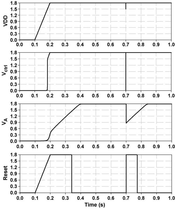
Fig. 4. Simulated transient responses during power-on and brown-out events.
