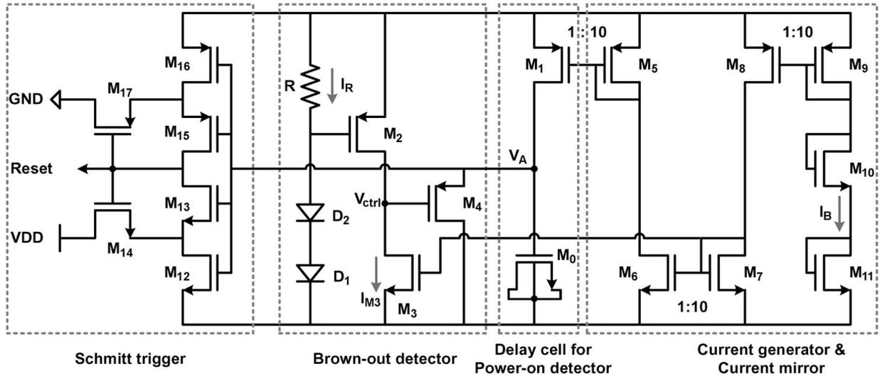
Fig. 3. Proposed POR circuit with BOR detection function.
