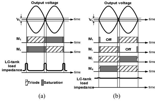
**Fig. 2.** Circuit operation in time domain: Conventional (a) and proposed voltage-bias differential LC-VCO (b).
