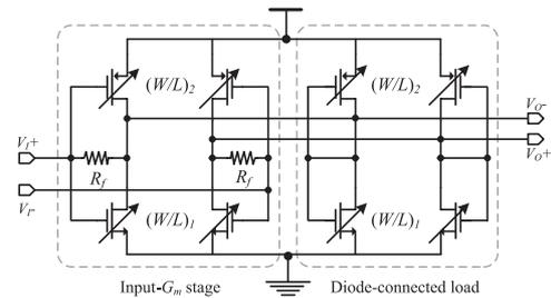
**Fig. 1** The current-reused-pseudo differential-pair based PGA architecture.
