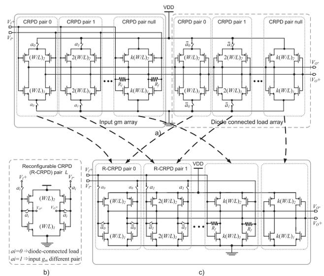
**Fig. 2** a) The proposed PGA with separated input- $G_m$  and load CRPD pairs. b) Schematic of configurable-CRPD pair. c) The proposed PGA schematic based on reconfigurable-CRPD pair.
