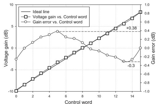
Fig. 4 Measured gain and gain-error versus control word.
