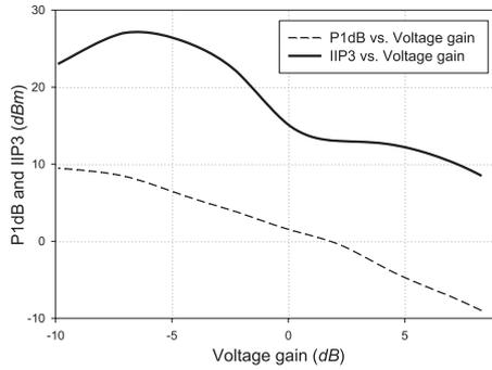
Fig. 5 Measured input P1 dB and IIP3 of the proposed PGA.
