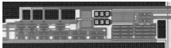
Fig. 3 Microphotograph of the proposed PGA chip.
