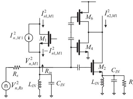
Fig. 2 The half of the proposed LNA for noise analysis.
