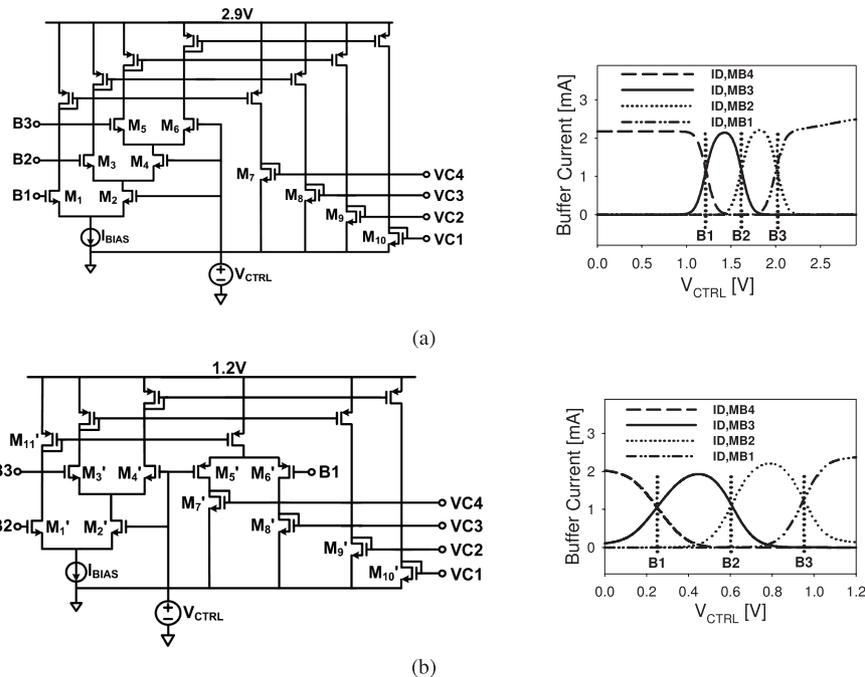
Fig. 2 ACC schematic and  $I_{D,MB1-4}$  vs.  $V_{CTRL}$  (a) reported [3], (b) proposed.
