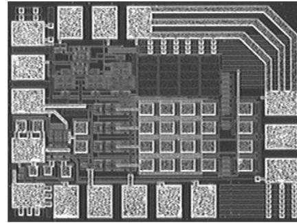
**Fig. 4** The die photograph of the proposed VGLNA for DVB-H.
