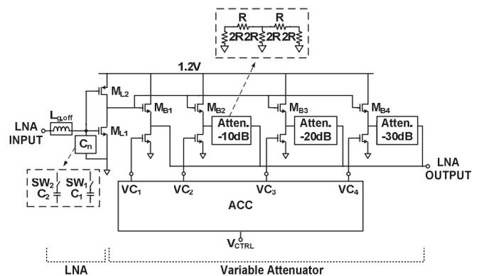
Fig. 1 Proposed frequency tunable VGLNA (bias is not shown).
